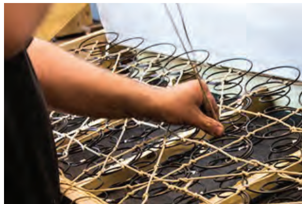
One of Grace Furniture's local craftsmen is creating a custom sofa using the traditional eight-way hand-tied construction technique, a nearly forgotten art.
